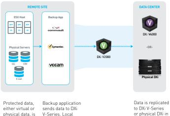
Data is replicated to DXi V-Series or physical DXi in data center for complete DR of remote site.
