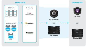
Protected data, either virtual or physical data, is sent to backup application. Backup application sends data to DXi V-Series or physical DXi. Local copy provides easy and fast restores. Data is replicated to DXi V-Series in the data center or to the cloud for complete DR of remote site.
